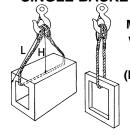
Most efficient when H is as large as L
